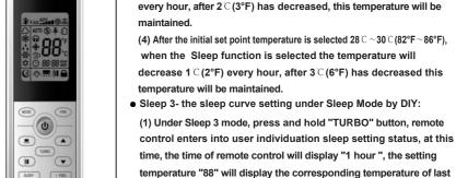
(2) Adjust ▲ and ▼ button, could change the corresponding setting temperature, after adjusted, press "TURBO "button for confirmation:
